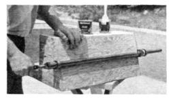
BODY for half-size 1901 Packard is made from half-inch plywood, glued and screwed at all joints and then clamped overnight.
