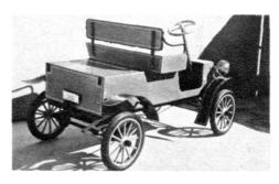
1901 PLATE, taillights and headlights are optional with builder. Note steering-shaft support, which is mounted to the dashboard.
