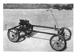
COMPLETED chassis and running gear with the brake pedal, brake rod, pedal-return spring, engine and drive assembly in place.
